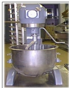
Figure 3: Planetary mixer for kneading
